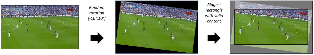
Figure 2: After the rotation is applied, corner spaces around the image are filled with default dark color. To end up purely with valid data containing the content of the image a crop is performed, representing the largest possible rectangle with content omitting the filled spaces created by rotation.
