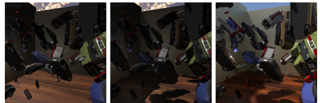
Figure 2: Image outputs with increasing levels of lighting realism. Left to right: Unity rasterizer without shadows, Unity rasterizer with shadow mapping, OctaneRender path-tracer.
