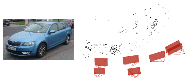
Figure 5: The best obtained result using COLMAP Structure from Motion tool for a sequence of images containing a stationary vehicle. Point cloud model (on the right) includes partially recognizable front part of the vehicle (especially its license plate) and the front wheel. Remaining parts of the vehicle are not included at all, or reconstructed incorrectly.
