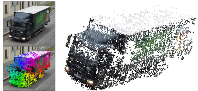
Figure 1: An example of points found by DeepMatching algorithm (left) and the corresponding result of 3D reconstruction of a passing truck (right).
