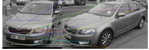
Figure 4: Example of found SIFT point correspondences on a static vehicle (30 best matches are shown). The vast majority of feature points is detected on the front part of the vehicle. Moreover, a significant number of incorrect matches can be observed.
