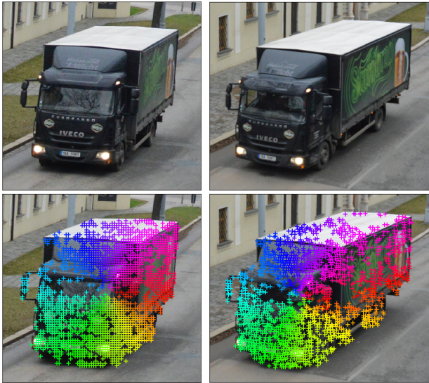
Figure 8: Correspondences for two images of a passing truck calculated using the DeepMatching algorithm and filtered with foreground masks.
