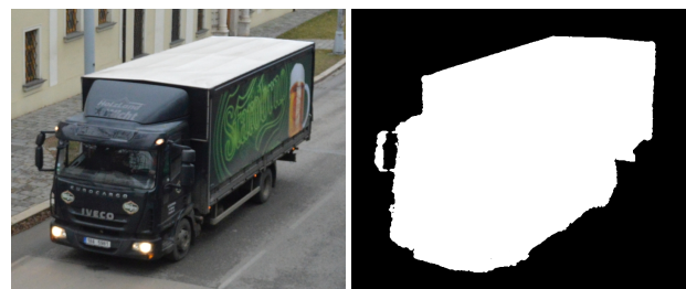
Figure 7: Original image of passing truck and its foreground mask.
