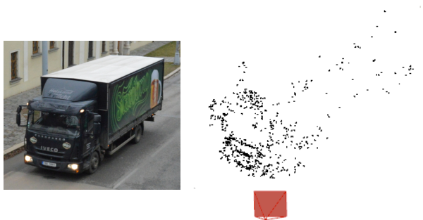
Figure 6: The best obtained result using COLMAP Structure from Motion tool for image sequence of passing vehicle. Resultant point cloud (on the right) contains recognizable front part of the truck.
