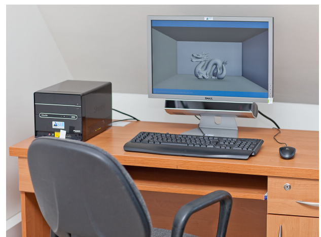
Figure 6: Apparatus used during evaluation and experiments. The RED250 eye tracker is located under the display screen.
