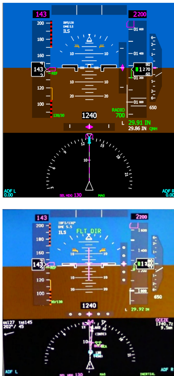
Figure 12: Comparison with the real system (top - our simulator, bottom - real system [5])
