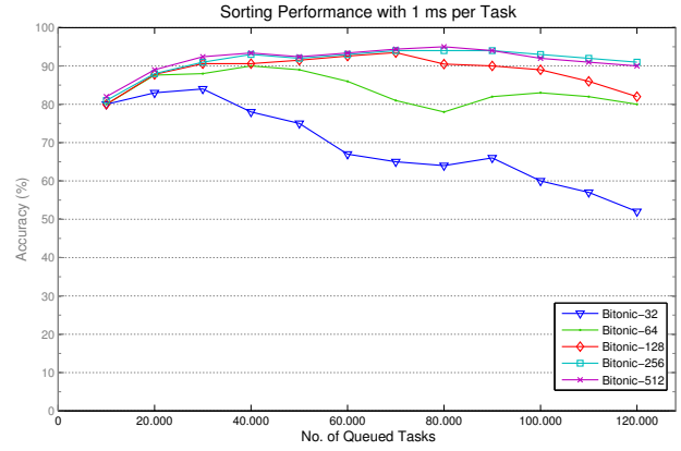
Figure 5: Evaluation of the algorithm performance for complex tasks with runtimes exceeding 1 ms. For smaller thread block sizes, we observe an early decline due to the increased effort for sorting a high number of entries with fewer threads. The highest recorded score of 95% is obtained using 512 threads.
