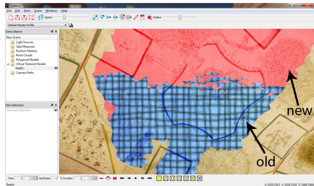
Figure 8: Visible artifacts while rendering in Scanopy resulting from simultaneous usage of the old (patterned) and the new version of tiles corresponding to a particular photograph.
