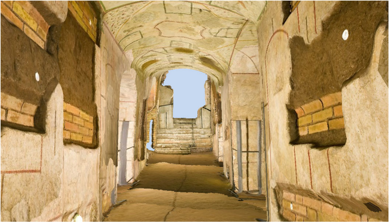
Figure 2: Part of the Domitilla Catacombs visualized using the unprocessed photographs. Especially on the floor the aforementioned artifacts are visible.
