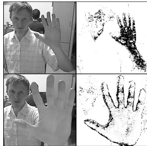
Figure 15: Example of bad back projection due to the luminance variation of the skin.
