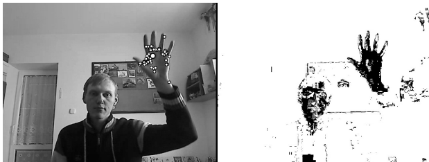
Figure 10: Result of histogram back projection with noise.
