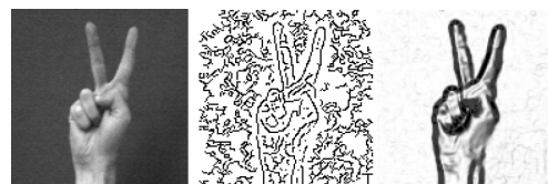
Figure 3: Original image, Canny detector, Oriented edge energy [15].
