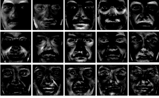
Figure 3: The eigenvectors, where the influence of illumination in the input images on the vectors with the biggest eigenvalues can be seen (the upper row), and the vectors with smaller eigenvalues, which represent features (the two bottom rows).
