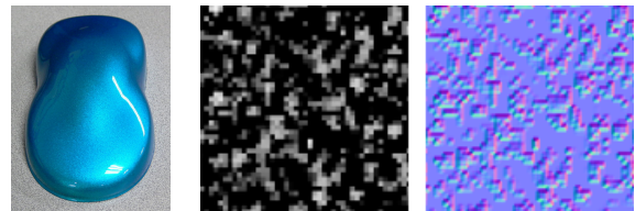
Figure 6: Left: Sparkling effect on an object coated with metallic paint. Right: An example of a texture representing the metallic flakes heightfield and the corresponding normal map.
