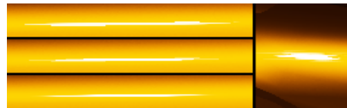
Figure 4: Zoom on a sharp specular highlight ( m_1 = 0.01 ) using tabulated D term with linear mapping (top), nonlinear mapping (middle) and the full evaluation (bottom). The right image shows a highlight when MIP-mapping is enabled on the texture which contains D .
