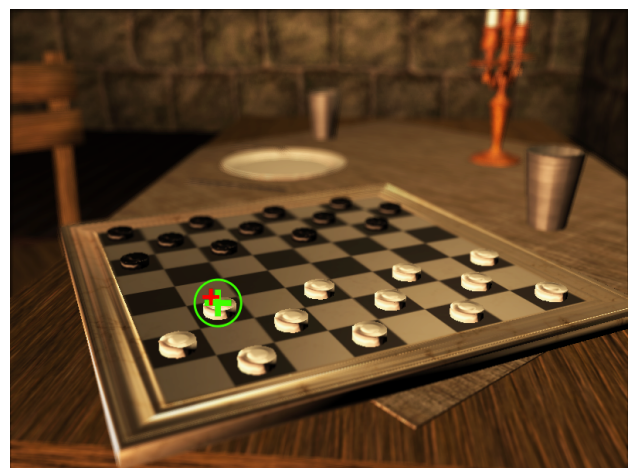
Figure 7: Example screens from our demo, containing on-screen feedback. Green crosshair represents the filtered, while red cross is the raw gaze point.
