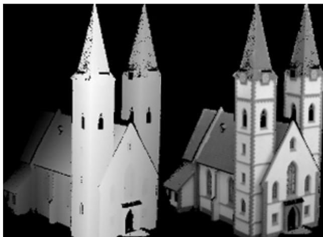
Figure 1: Example range image and co-registered reflectance image obtained with the Minolta Vivid 900.
