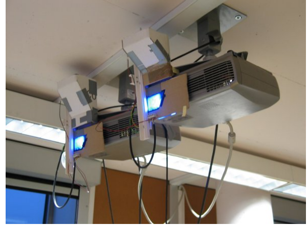
Figure 2: LC-Shutters mounted on the projector casing with cooling fan.
