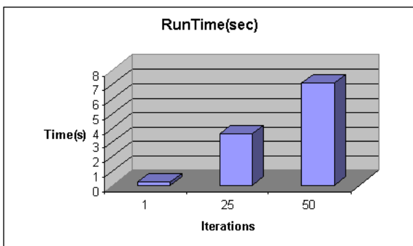
Figure 7: Running time of the proposed algorithm (pbuffer size is 512 \cdot 512 )
